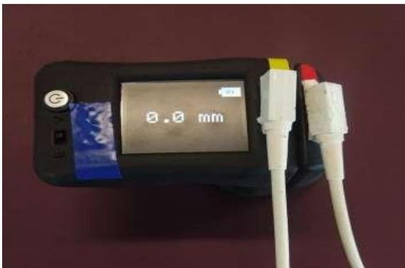
**Figure B:** The Mobil-Aider with Trakstar electromagnetic markers attached
