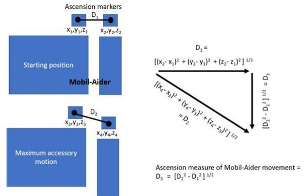
**Figure D:** Calculation of maximum Mobil-Aider distance using absolute position of 2 Ascension markers in the x, y and z coordinate planes
