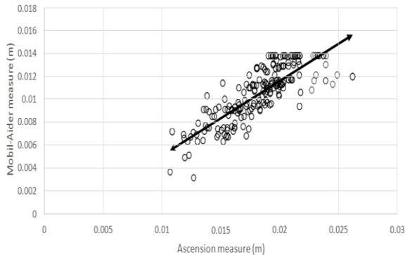
**Figure E:** Relationship between joint accessory movement measurements obtained by the Ascension system (x axis) and the Mobil-Aider (y axis)
